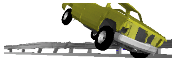
-Strong-Post Guardrail with 150-mm Curb- F.E. Simulation of a 2000P
